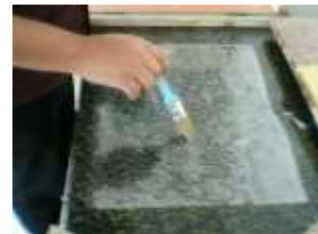
(c) Application of first resin coat
